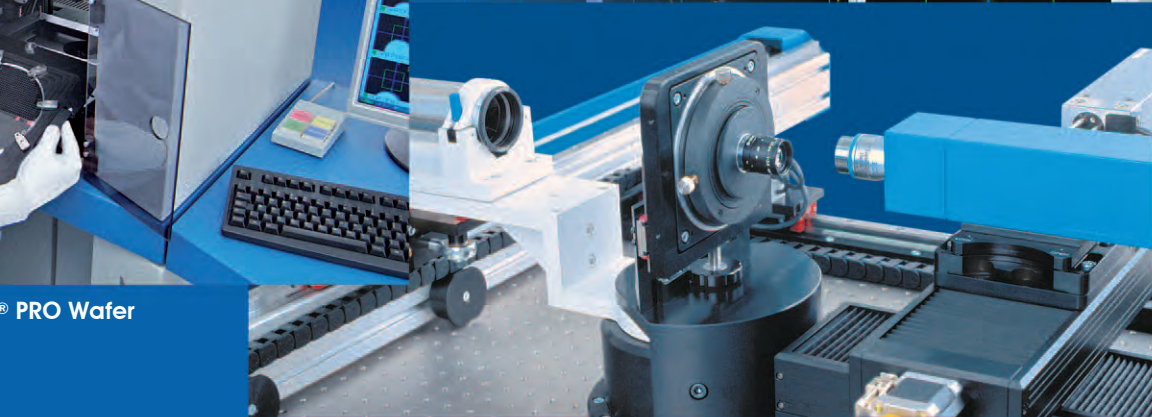
Measurement of CCD-Objective lenses
