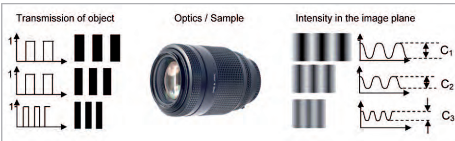
Fig. 1 A perfect grid pattern is imaged through the sample into the image plane
