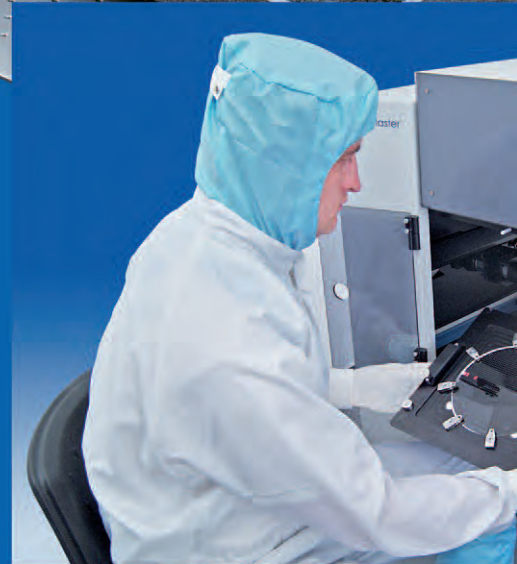
Testing wafer level lenses with ImageMaster®
